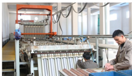
自动电镀线 Automatic electroplating production line
