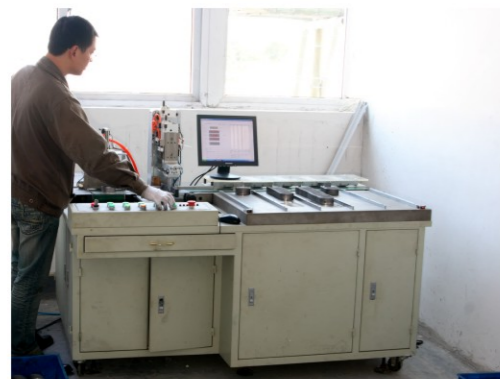
自动壁厚分选仪 Automatic thickness sorting machine
