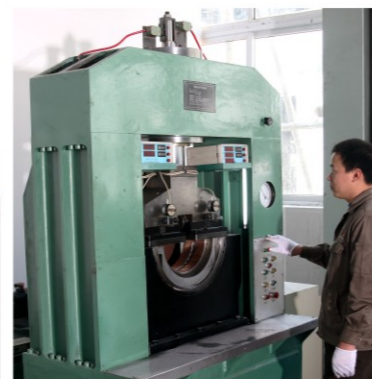
双面加载高度测量仪 B method crush high measure machine
